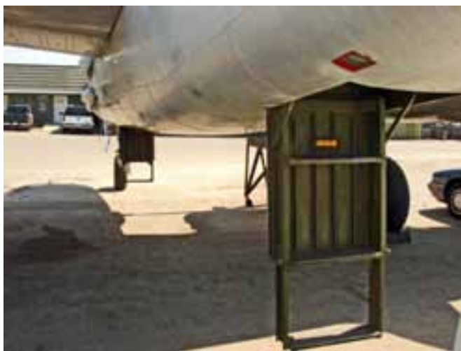
B-25 crew entry hatch and ladder assembly (jettisoned as escape hatch) D. Poissant photo
